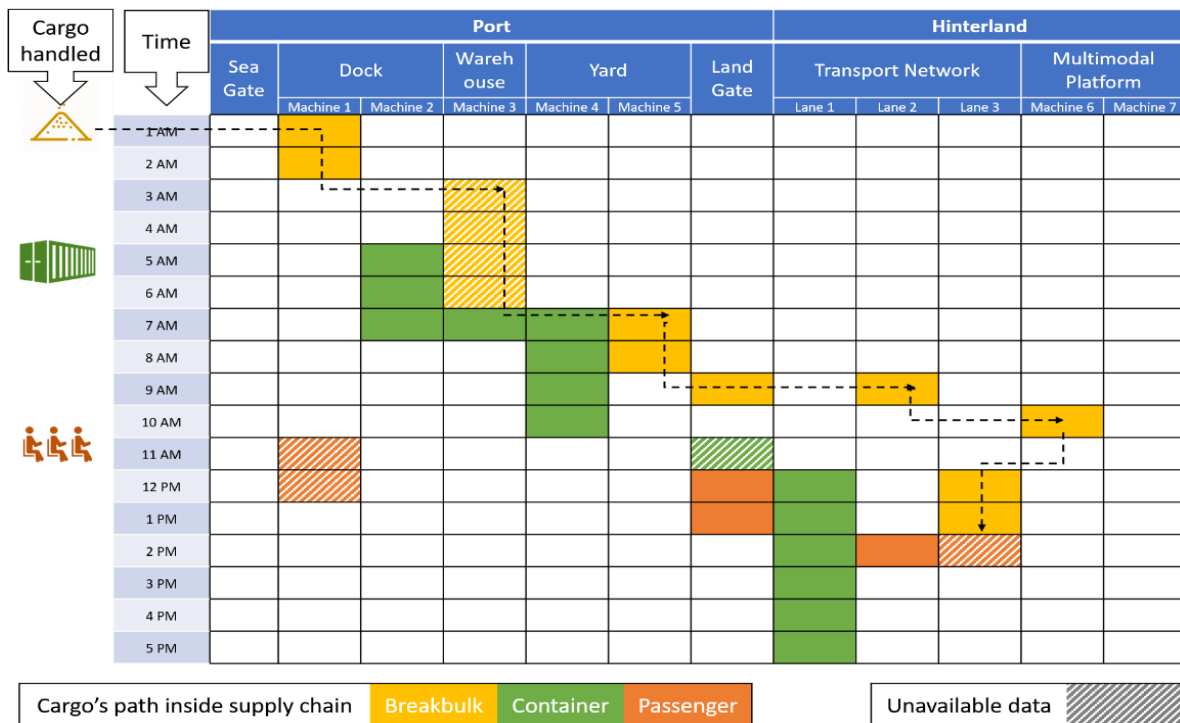
Figure 8: Activity's data structure consists in handled cargo's data projected on time and machine/space axes
